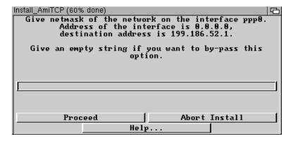
With every IP address you must supply a netmask. It's usually quite easy for AmiTCP to figure out this address, so you can leave this option blank. However, if for some reason you have to enter a netmask then check with your ISP, though 255.255.0 is a good bet.
