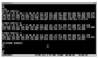
At the top of the screen you can see the active settings for this modem. Further down you can see that the modem has two memory banks where it can store alternative settings. It can even store frequently called phone numbers. Let's go through some of the most important AT commands and S-Registers. The commands shown to the right have been tested only on Supra modems but most modern modems should use the same commands. Again, check with your manual for any small differences.
