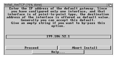
The default gateway is the machine to which your Amiga will forward all Internet destined packets. Because you have a point-to-point link to your ISP, all of your IP packets must go to the machine at the other end of your modem link, so usually this remote machine is the default gateway.
