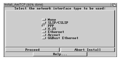
TCP/IP can run over a variety of different network types. It is possible to install Ethernet or Arcnet cards in a number of Amigas and network them together locally. However, if you are simply using a modem to connect to the Internet then you need a piece of software under AmiTCP to talk to your modem. This is usually SLIP, CSLIP or PPP. The most popular these days is PPP, using the aforementioned dynamic addressing. Click on whichever protocol your ISP has told you to use.
