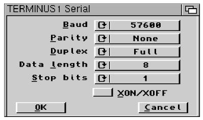
These extra bits are used for clocking information. The two modems don't know whether your eight bits are going to be ones or zeros, but if they can rely on start and stop bits always being present then over long periods of time they will never lose synchronisation with each other. If the two modems lost track of which bits were which and got confused about what was the start of a particular data byte, you would just get complete garbage coming out at both ends.
